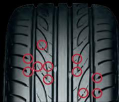
Non-penetrating lug grooves aim to reduce noise. The blocks increase the stiffness to improve the direct handling and to reduce friction.
