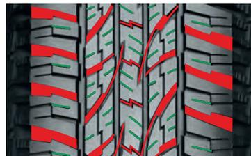
The optimised allocation of the lug grooves help to beat down off-road surfaces to support traction.
